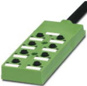
Sensor/actuator box, Connection method: M12 socket Plastic, Number of slots: 8, Number of positions: 5, Slot assignment: Double, Status indication: Yes, pnp; Master cable connection: Fixed connection 180°, PUR halogen free, Cable length: 5 m, Shielding: No
