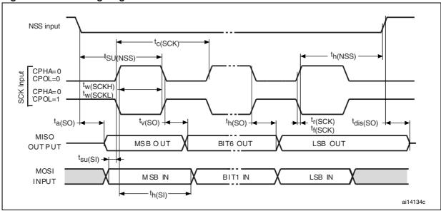
Figure 28. SPI timing diagram - slave mode and CPHA = 1<sup>(1)</sup>
