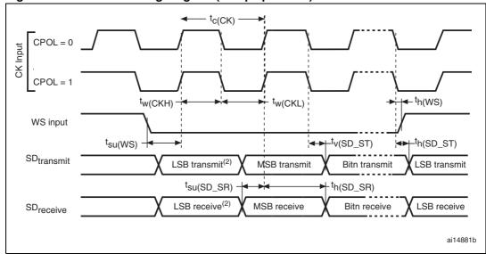
Figure 30. I2S slave timing diagram (Philips protocol)
