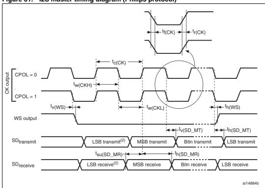
Figure 31. I2S master timing diagram (Philips protocol)
