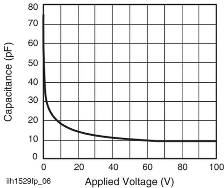
Fig. 6 - Switch Capacitance vs. Applied Voltage
