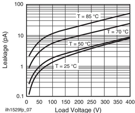
Fig. 7 - Leakage Current vs. Applied Voltage
