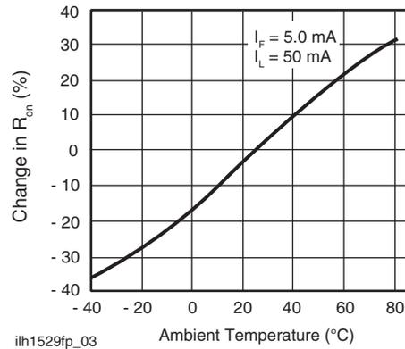
Fig. 3 - On-Resistance vs. Temperature
