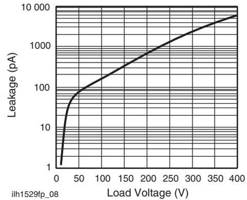
Fig. 8 - Leakage Current vs. Applied Voltage
