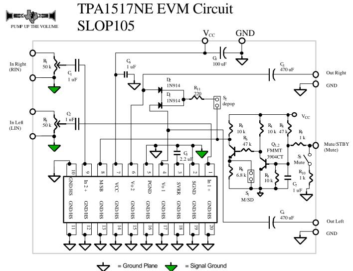
Figure 2 - Schematic of 1517NE EVM
