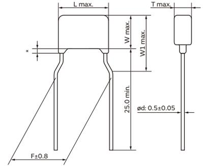
\* Coating extension does not exceed the end of the lead bend.
