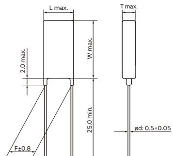
· Lead Wire: Solder Coated CP Wire
