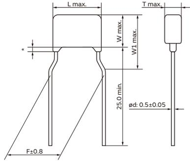
\* Coating extension does not exceed the end of the lead bend.
