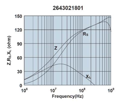
Impedance, reactance, and resistance vs. frequency.
