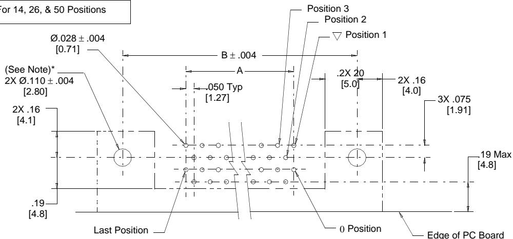
\*Note: Plated-through mounting holes for .062 [1.57] PC board thickness
