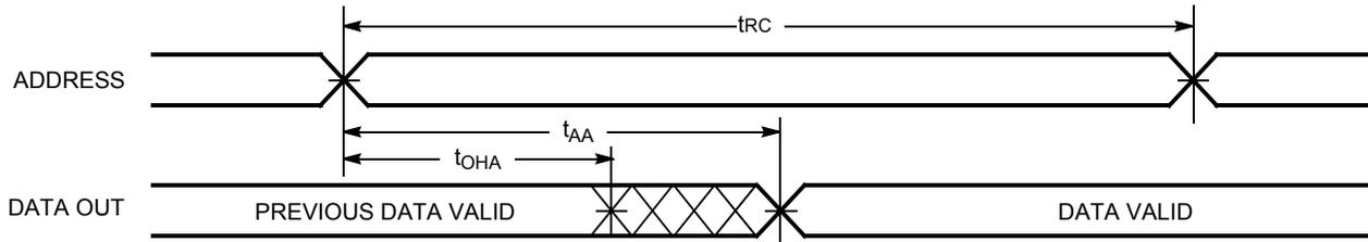
Figure 6. Read Cycle No. 2 ( $\overline{OE}$  Controlled) [15, 16]
