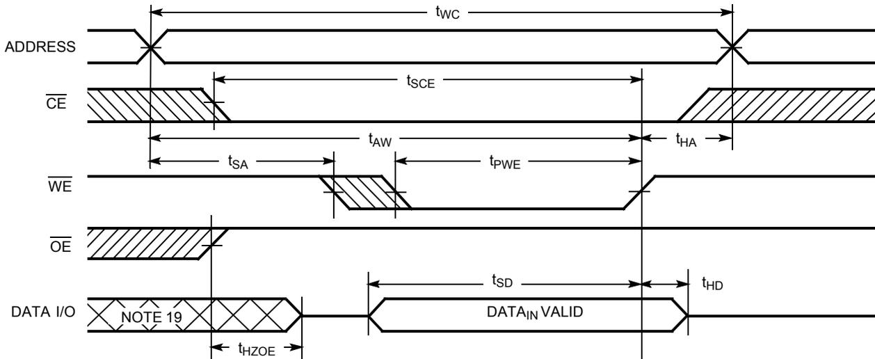
Figure 8. Write Cycle No. 2 ( $\overline{WE}$  Controlled,  $\overline{OE}$  LOW) [18]
