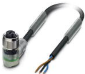
Sensor/actuator cable, 3-position, PUR/PVC, gray RAL 7001, free cable end, on Socket angled M12, A-coded, with 2 LEDs, cable length: 5 m
