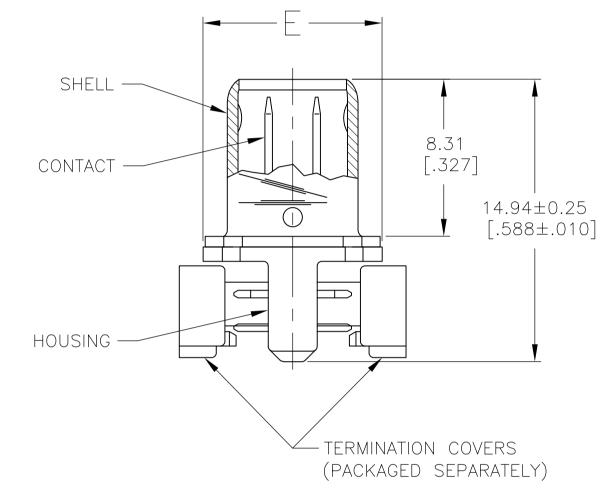
HOUSING AND TERMINATION COVERS: THERMOPLASTIC, UL94V-O RATED, COLOR BLACK. SHELL: STEEL. PIN CONTACTS: PHOSPHOR BRONZE.
