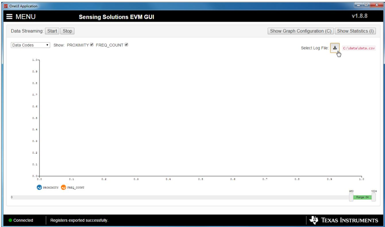
**Figure 1-27. Select Log File Button on Data Streaming Page**
