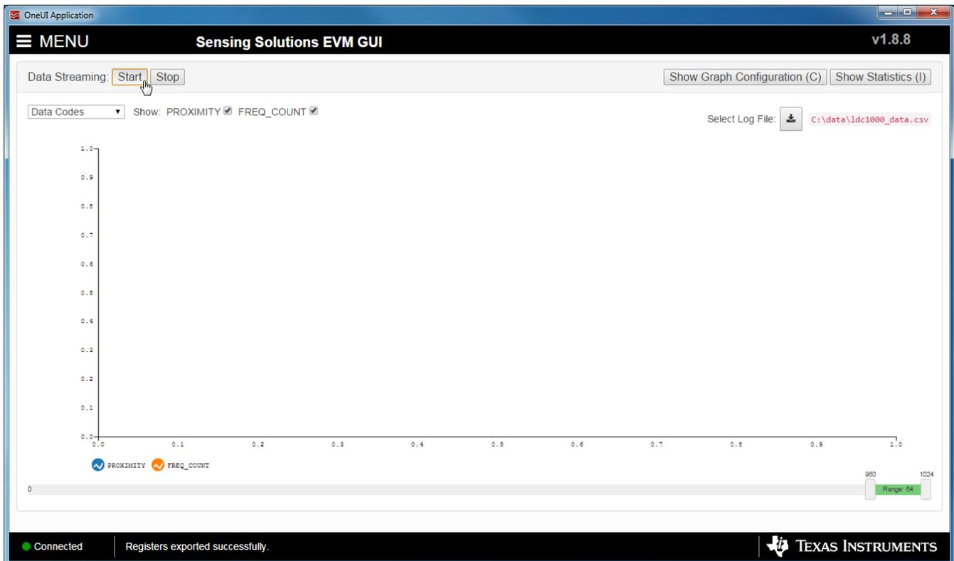
Figure 1-28. Start Button on Data Streaming Page
