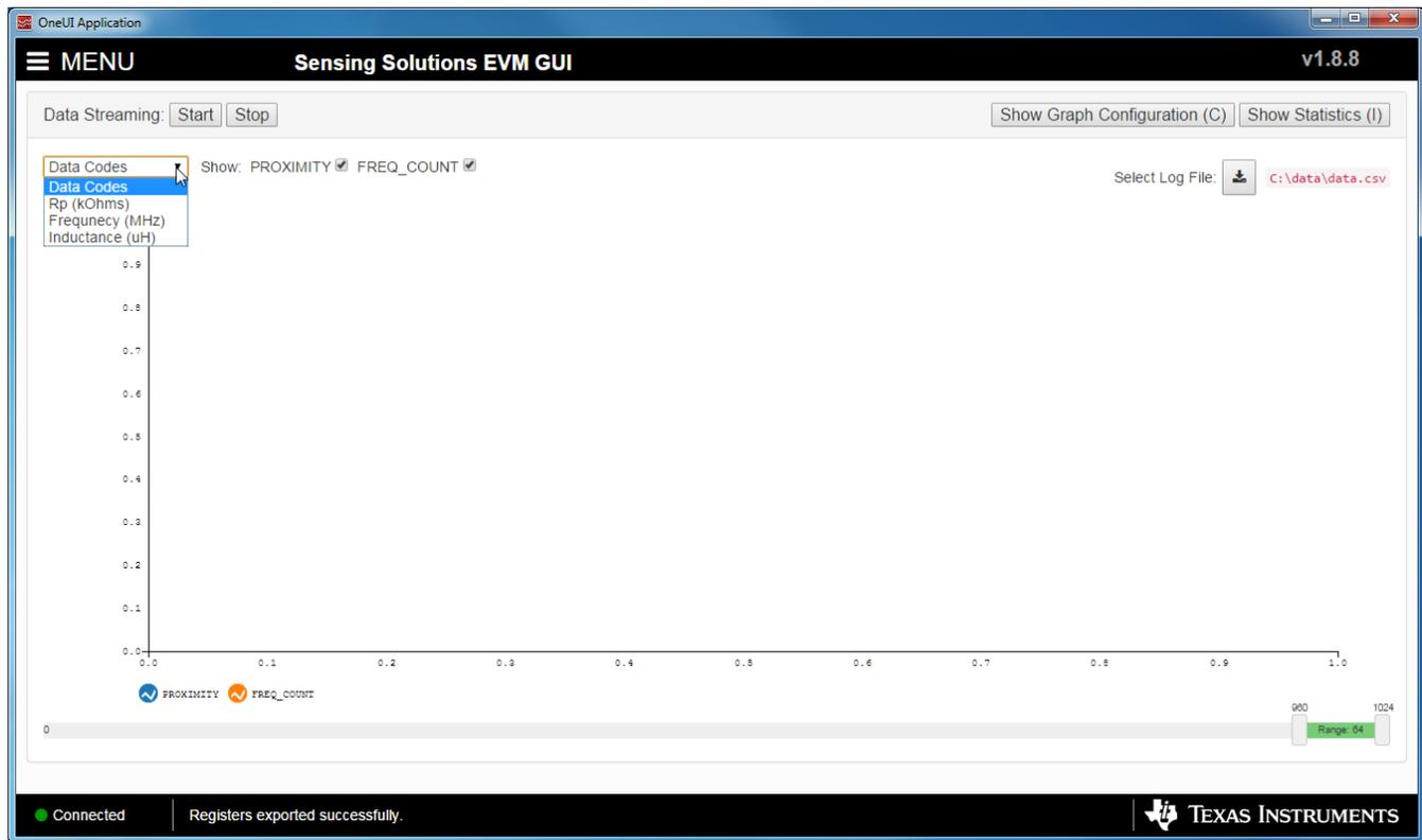
**Figure 1-26. Select the Data Graph on Data Streaming Page**
