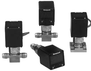
With space at a premium in semiconductor gas distribution systems, the Series TLD pressure transducer with local display offers an integrated solution that reduces the overall height of the transducer/display assembly to as little as 3.5 in [88.9 mm]. To accomplish this, the transducer's signal amplifier is mounted within the display, with the added benefit of zero and span adjustments conveniently located on the LED display face.
