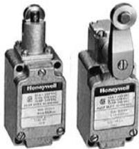
LS Series compact limit switches are carefully designed for accurate repeatability under the most stringent conditions. Compact size and field adjustable features greatly extend the flexibility of these switches. Heads may be positioned at 90° increments. Side rotary models can be adjusted for clockwise and/or counter-clockwise operation. Actuators can be set and locked in any position through 360°.
