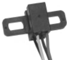
The S-180 Series consists of a gallium arsenide IRED and silicon phototransistor mounted in a rigid one-piece polycarbonate housing. All electrical options are available with either PCB mount or 457,0 mm (18.0 in) minimum length wire termination (26 AWG type UL 1429)
