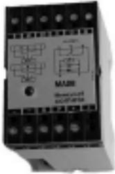
The FF-MADB24RB is a small and versatile power supply usually used with the ultrasonic distance sensors, but may be used for any purpose. The power supply accepts 115 or 230 Vac input, is regulated to 24 Vdc. An internal SPDT relay may be triggered by NPN or PNP sensor output.
