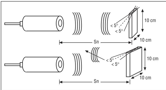
Figure 2: Effect of target inclination on the measurement
