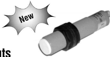
The new 944 series are microprocessor controlled and fully programmable by teach-in, with the simple pressing of a button. They offer analogue and two switching outputs through a standard M-12, 5-pin connector. All the models are IP67 with chemical-resistant body and epoxy face. Parameters are stored in non-volatile memory.
