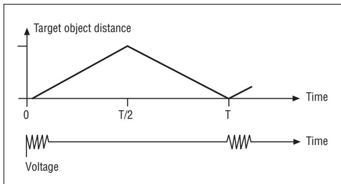
**Figure 1** shows the elapsed time of the acoustic pulse. The diagram shows how the pulse travels from the transducer to the target, is reflected at time  $T/2$ , and reaches the transducer at time  $T$ . Below is a diagram of the voltage at the ultrasonic transducer. Elapsed time  $T$  is directly proportional to object distance  $a$ .  $a = cT/2$ , where  $c$  is the velocity of sound.
