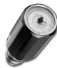
The Series 940 Torque Watch accurately measures torque in values that range from 15.0 to 200 oz/in. A 3/8 inch keyed chuck and 3/8 inch square socket driver adapter provide a simple means of coupling to the device under measurement.
