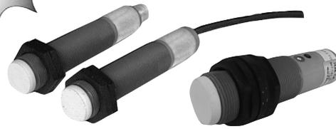
The new 940/947 Series is microprocessor controlled, can be set up quickly and are fitted with epoxy transducers. All the housings are sealed to IP67. The retroreflective versions allow detection of any kind of target without any dead zone. They work with a reflector target.
