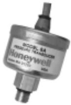
The harsh duty SA pressure transducer has a water resistant, stainless steel case for complete protection from harsh environments. Internal hermetic sealing is used to provide measurement from absolute pressures (psia) or pressures referenced to a sealed chamber (psis). Underwriters Laboratories has approved the SA as a component in float and pressure-operated motor controllers (File #E93356).
