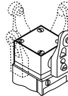
Momentary action switches can be factory assembled for operation in one direction only and/or with the shaft facing the rear or either side. Contact Honeywell for more information.
