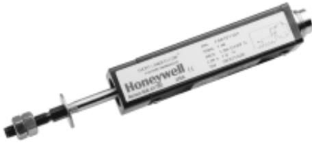
The Short Longfellow is frequently used for measuring linear position or displacement up to 6 inches (152,4 mm) on a wide variety of manufacturing and process equipment. The mechanical design of the unit's front bearing, anodized extruded aluminum housing, stainless steel shaft and precious metal wipers are suitable for a factory's harsh environment.
