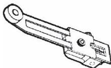
**Operating radius/length:** 1.5 in to 3.5 in (38,1 mm to 88,9 mm)
