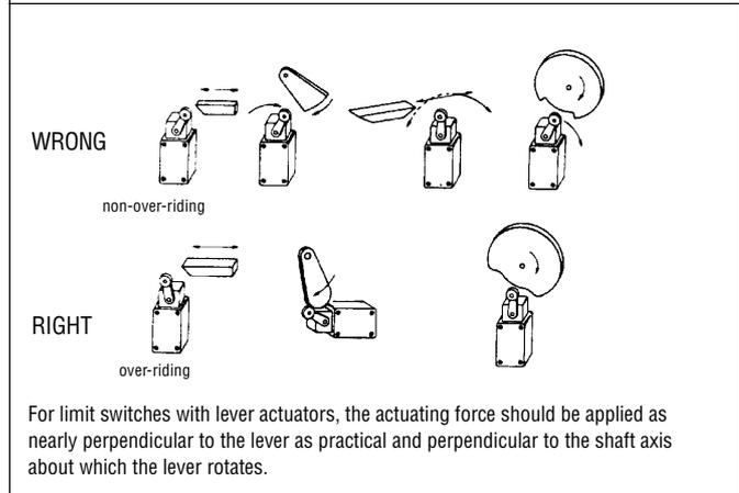
For limit switches with lever actuators, the actuating force should be applied as nearly perpendicular to the lever as practical and perpendicular to the shaft axis about which the lever rotates.
