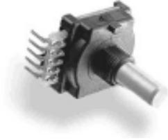
The 510 Series controls are manually operated, rotary, mechanical encoders that provide a two-bit gray code for relative reference applications and a four-bit gray code for absolute electrical reference applications. The "L" channel leads the "R" channel by 90° electrically in the CW position. It features continuous electrical travel and has a rotational life of more than 100,000 shaft revolutions with a positive detent feel.
