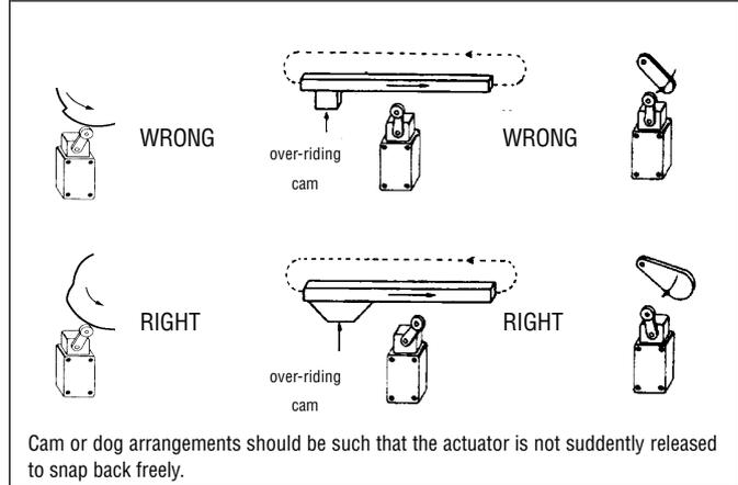
Cam or dog arrangements should be such that the actuator is not suddenly released to snap back freely.
