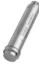
The BL pressure transmitter has a conventional 4 mA to 20 mA output and is available with accuracies to 0.25%. It has Factory Mutual approval as an intrinsically safe device for use in hazardous areas. Class I, Division I, Groups A through G (when used within approved barriers).
