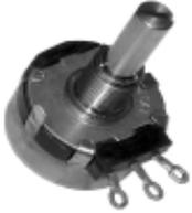
The 380 Series "Quiet One" is a 2-watt conductive plastic potentiometer offering superior dynamic noise and a long rotational life. It meets MIL-R-94 specifications where applicable.
