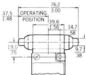
LSG contact transfer is maintained after either plunger is operated. Operation of other plunger resets switch.
