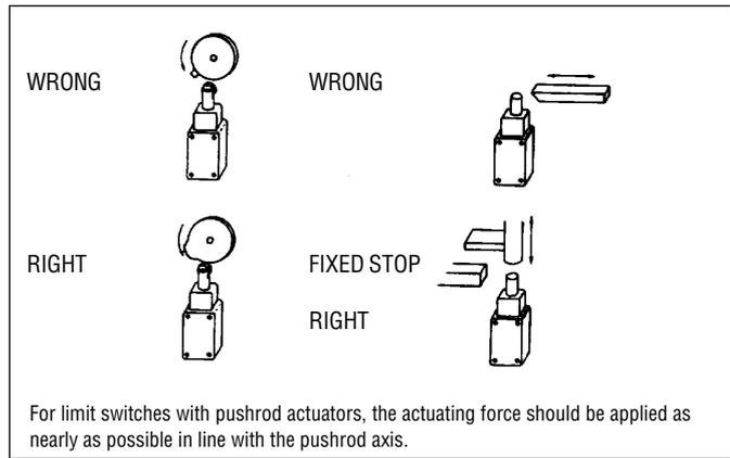
For limit switches with pushrod actuators, the actuating force should be applied as nearly as possible in line with the pushrod axis.
