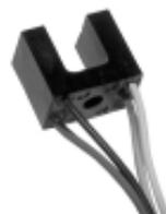
The S-510 Series consists of a gallium arsenide IRED and silicon phototransistor mounted in a small injection-molded housing. An IR-opaque housing is offered for applications where high levels of ambient infrared radiation may be present and an IR-transparent housing for applications requiring protection from dust and dirt in the apertures. This series is also available with 305,0 mm (12.0 in) minimum length flexible wire leads.
