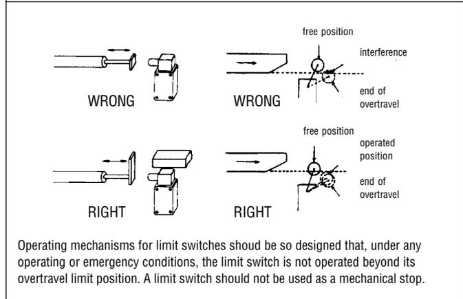
Operating mechanisms for limit switches should be so designed that, under any operating or emergency conditions, the limit switch is not operated beyond its overtravel limit position. A limit switch should not be used as a mechanical stop.
