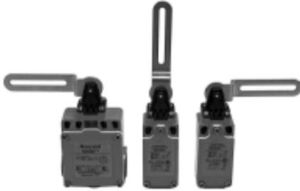
The Hinge Mount Safety Limit Switch is designed for use on machine access doors as an alternative solution to key operated interlocks and safety limit switches. When the access door is opened, a follower pin (not supplied) slides down the slot in the actuator lever, forcing the actuator lever to rotate and positively open the NC safety circuit to shut off the machine. Closing the access door rotates the actuator lever to the reset position, closing the NC safety contacts.
