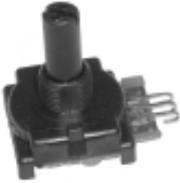
The 575 Series conductive plastic potentiometer offers a smooth feel and robust construction, with a thermoplastic housing, bushing, and shaft. Terminals are solder-hook style for panel mounting. No hardware is included.
