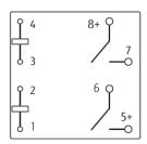
Relay contact terminals have polarity.
