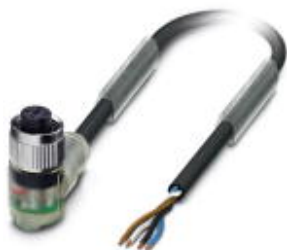
Sensor/actuator cable, 4-position, Variable cable type, free cable end, on Socket angled M12, A-coded, with 2 LEDs, cable length: Free input (0.2 ... 40.0 m)
