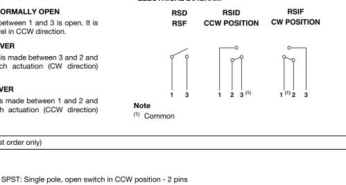
RSIDSPDT: Single pole, changeover switch in CCW position - 3 pinsRSIFSPDT: Single pole, changeover switch in CW position - 3 pins
