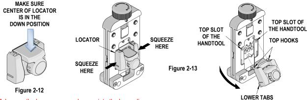
**Note**: Make sure the longer screw only goes into the lower dies.
