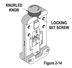
1. Loosen the locking set screw located just below the knurled knob at the top of the Power Crimp Head. See Figure 2-14.
