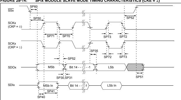
FIGURE 28-14: SPIX MODULE SLAVE MODE TIMING CHARACTERISTICS (CKE = 1)
