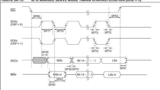
FIGURE 28-13: SPIX MODULE SLAVE MODE TIMING CHARACTERISTICS (CKE = 0)
