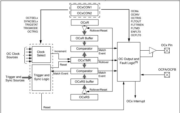
Note 1: The OCx outputs must be assigned to an available RPn pin before use. Please see Section 10.4 "Peripheral Pin Select" for more information.
