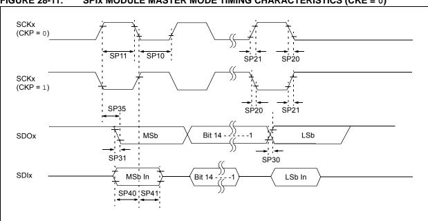
FIGURE 28-11: SPIX MODULE MASTER MODE TIMING CHARACTERISTICS (CKE = 0)
