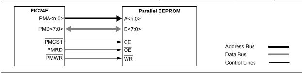
FIGURE 18-11: PARALLEL EEPROM EXAMPLE (UP TO 15-BIT ADDRESS, 16-BIT DATA)
