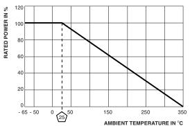
Derating is required for ambient temperatures above 25 °C per the above graph.
