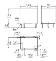
Dimensions (thickness and width) of terminal is measured before pre-soldering.
