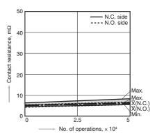
7-(4). Electrical life test (Lamp load)
