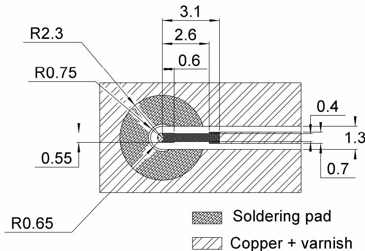
Substrate: RO4350 thickness 0.254mm, with copper layer 35 $\mu$ m on both sides:
