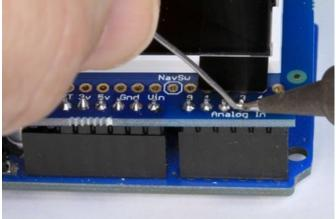
And Solder! Solder each pin to assure good electrical contact.
