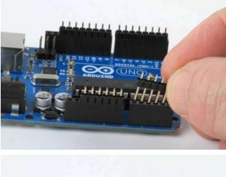
Insert the Headers into an Arduino To align the header strips for soldering, insert them (long pins down) into the headers of an Arduino.
