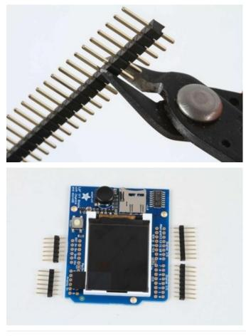
Cut the Header Sections Cut the breakaway header strip into sections to fit the holes on the edge of the shield. You will need 2 sections of 6-pins and 2 sections of 8 pins.
