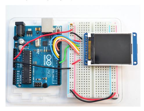
Wiring up the display in SPI mode is pretty easy as there's not that many pins! We'll be using hardware SPI, but you can also use software SPI (any pins) later. Start by connecting the power pins
