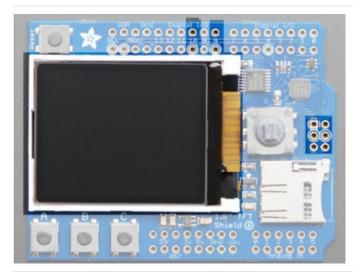
In the center is the 1.8" TFT display. This display is full color (16-bit RGB), 128x160 pixels, and has a backlight. The display receives data over SPI plus two pins:
