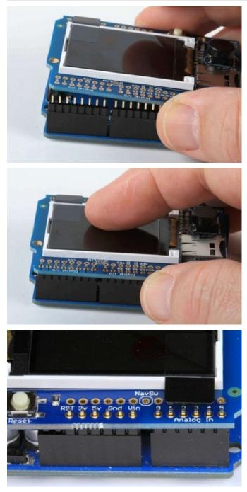
Add the Shield Place the shield over the header strips so that the short pins stick up through the holes.
