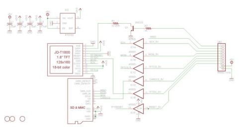
For the level shifter we use the CD74HC4050 which has a typical propagation delay of ~10ns
