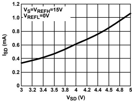
FIGURE 3. DIGITAL SUPPLY VOLTAGE vs DIGITAL SUPPLY CURRENT
