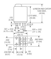
Mounting code 5 Printed circuit terminals
