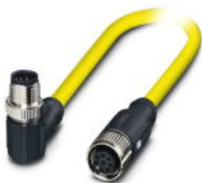
Sensor/actuator cable, 8-position, PVC, yellow, shielded, Plug angled M12 SPEEDCON, coding: A, on Socket straight M12 SPEEDCON, coding: A, cable length: 0.5 m
