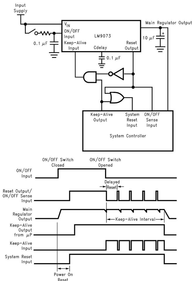
**Figure 19. Simple Logic Configuration to Provide ON/OFF Sensing**
