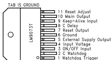
Figure 1. 11-Lead TO-220 (Top View)
