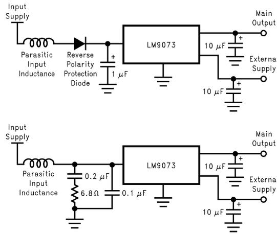
Figure 20. Input Bypassing
