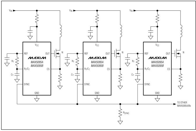
Figure 9. Synchronization of MAX5095A/MAX5095B
