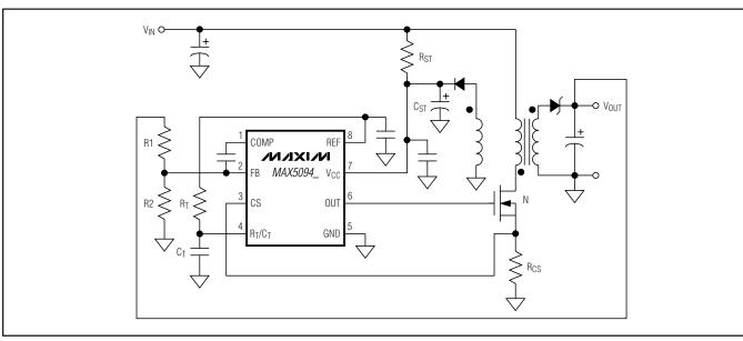
Figure 6. MAX5094\_ Typical Application Circuit (Nonisolated Flyback)
