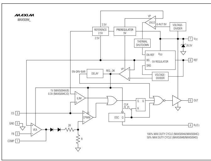
Figure 1. MAX5094\_ Functional Diagram
