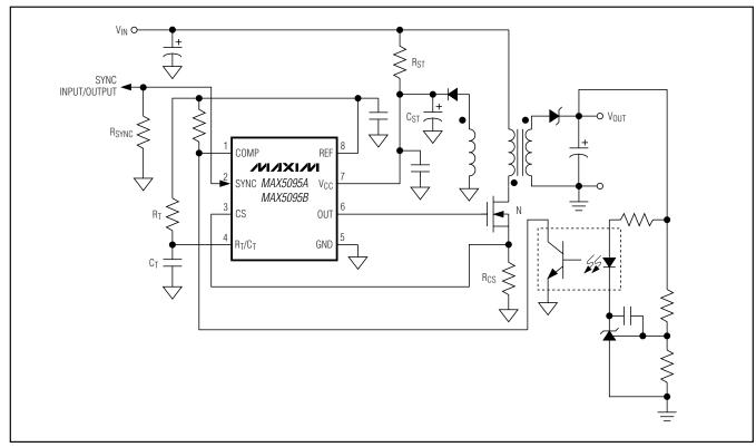
Figure 7. MAX5095A/MAX5095B Typical Application Circuit (Isolated Flyback)
