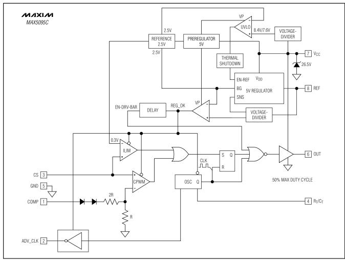
Figure 3. MAX5095C Functional Diagram
