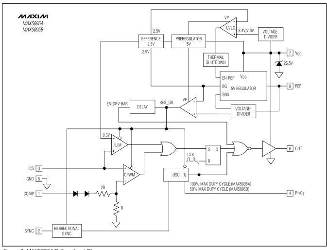
Figure 2. MAX5095A/B Functional Diagram
