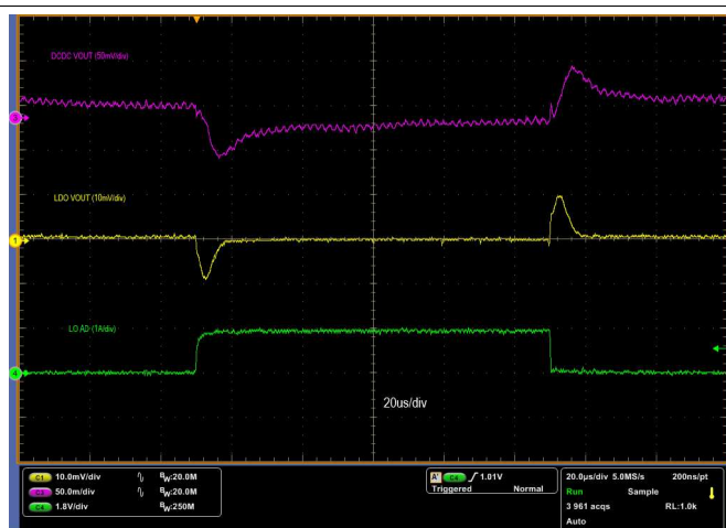
V_{IN} = 5\text{ V} , V_{OUT} = 2.1\text{ V} , LDO_{V(out)} = 1.8\text{ V} , Load = 1 A to 2 A
