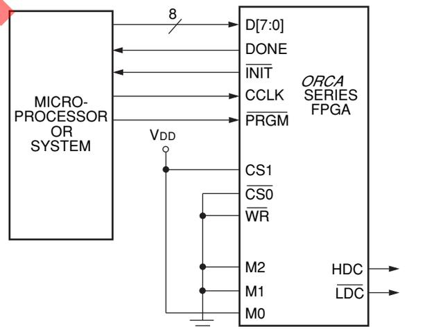
Figure 62. Slave Parallel Configuration Schematic
