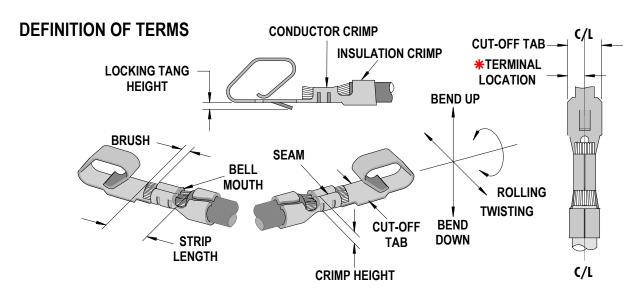
\*Terminal is to be centrally located between the two (2) cut-off tab edges by one half of the total cut-off tab tolerance.
