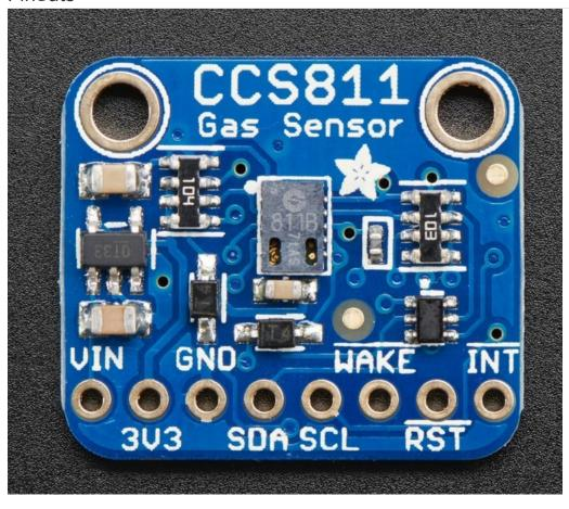
This sensor has 2 mounting holes and one header breakout strip.
