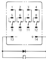
(Check the coil polarity when wiring and wire all connections correctly.)
