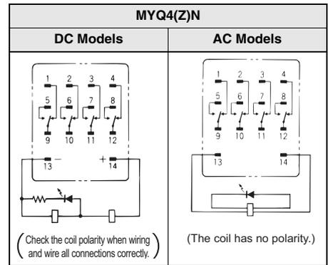
**Note:** 1. An AC model has coil disconnection self-diagnosis.
