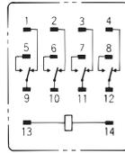
(The coil has no polarity.)
