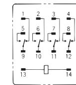
(The coil has no polarity.)
