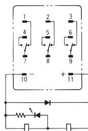
(Check the coil polarity when wiring and wire all connections correctly.)
