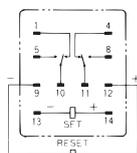
**Note:** Pay close attention to the set coil and reset coil polarities. If the connections are not correct, unintended operation may occur.
