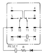
**Note:** R is a resistor for ampere-turn correction. This resistor is built-in to 50-VAC and higher models. (The coil has no polarity.)
