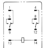
(The coil has no polarity.)
