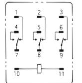
(The coil has no polarity.)
