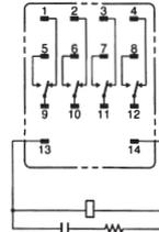
(The coil has no polarity.)
