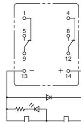
**Note:** For the DC models, check the coil polarity when wiring and wire all connections correctly.
