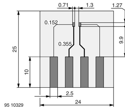
Fig. 3 - Board for  $R_{thJA}$  Definition (in mm)
