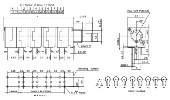
Model P09x5N (Top Adjust, PCB pins, up to 2 gangs)
