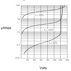
Instantaneous Reverse Leakage Current - MicroAmperesversus Percent Of Rated Peak Reverse Voltage - Volts
