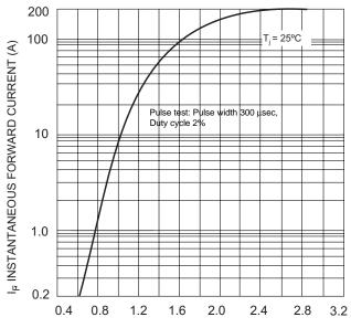
Instantaneous Forward Current - Amperes versus Instantaneous Forward Voltage - Volts
