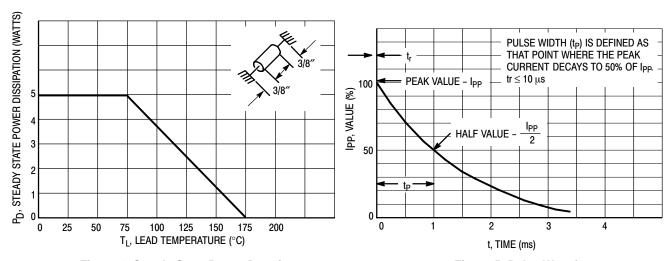
Figure 4. Steady State Power Derating
