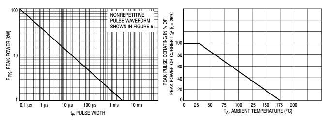
Figure 1. Pulse Rating Curve
