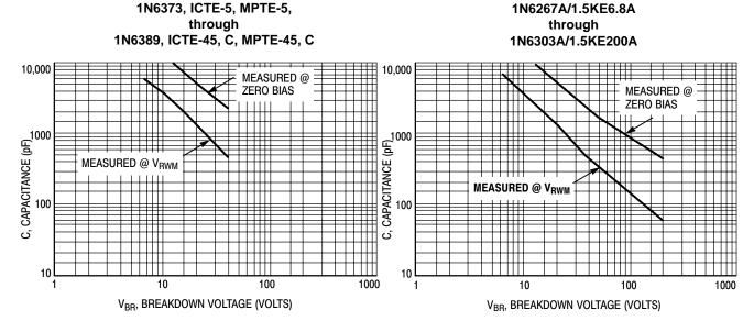
Figure 3. Capacitance versus Breakdown Voltage
