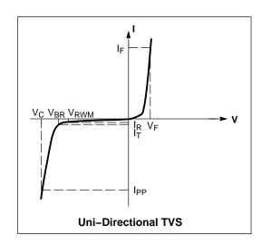
**ELECTRICAL CHARACTERISTICS** ( $T_A = 25^{\circ}C$  unless otherwise noted,  $V_F = 3.5 \text{ V Max.}$  @  $I_F$  (Note 3) = 100 A)
