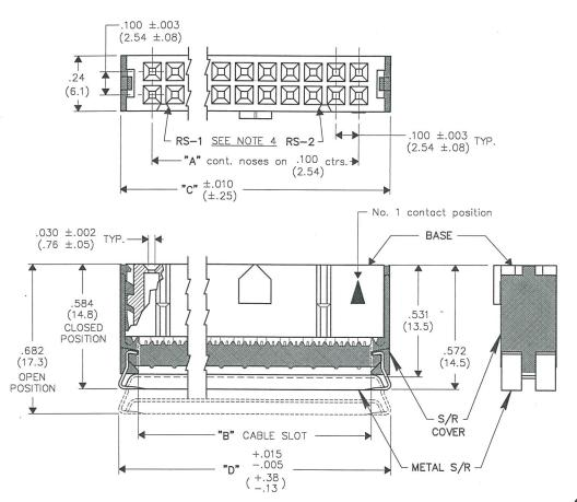
DIMENSIONS IN INCHES (MILLIMETERS) DO NOT SCALE DRAWING .....
