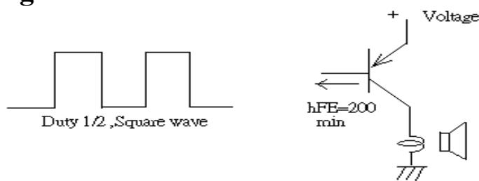
**The base current  $I_b$  should be high enough so that it saturates the collector current of the transistor with the CB load.**
