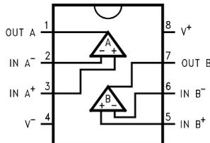
**Figure 1. 8-Pin PDIP/SOIC - Top View**
