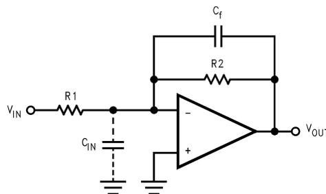
**Figure 58. Cancelling the Effect of Input Capacitance**
