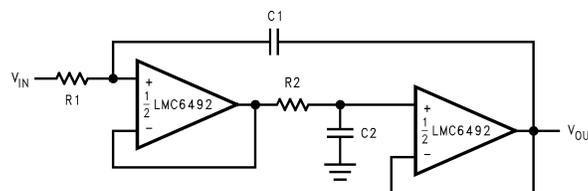
$$R_1 = R_2, C_1 = C_2; f = \frac{1}{2\pi R_1 C_1}; \text{Damping Factor} = \frac{1}{2} \sqrt{\frac{C_2}{C_1}} \sqrt{\frac{R_2}{R_1}}$$
