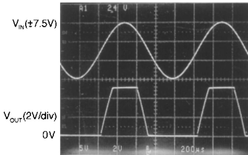
Figure 56. A ±7.5V Input Signal Greatly Exceeds the 5V Supply in Figure 57 Causing No Phase Inversion Due to R<sub>I</sub>
