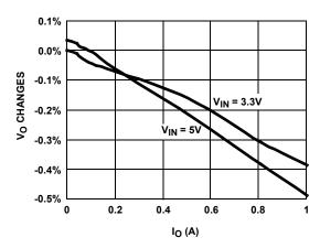
FIGURE 6. LOAD REGULATIONS (PWM MODE)
