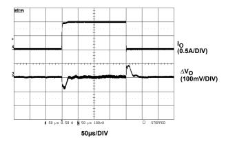
FIGURE 20. PWM LOAD TRANSIENT RESPONSE (0A TO 1A)
