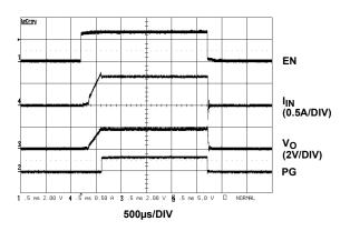
FIGURE 14. ENABLE AND SHUT-DOWN
