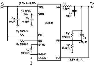
$* V_0 = 0.8V * (1 + R_1 / R_2)$
