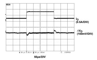
FIGURE 21. PWM LOAD TRANSIENT RESPONSE (0.25A TO 0.75A)
