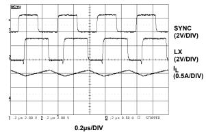
FIGURE 17. EXTERNAL SYNCHRONIZATION TO 2MHz
