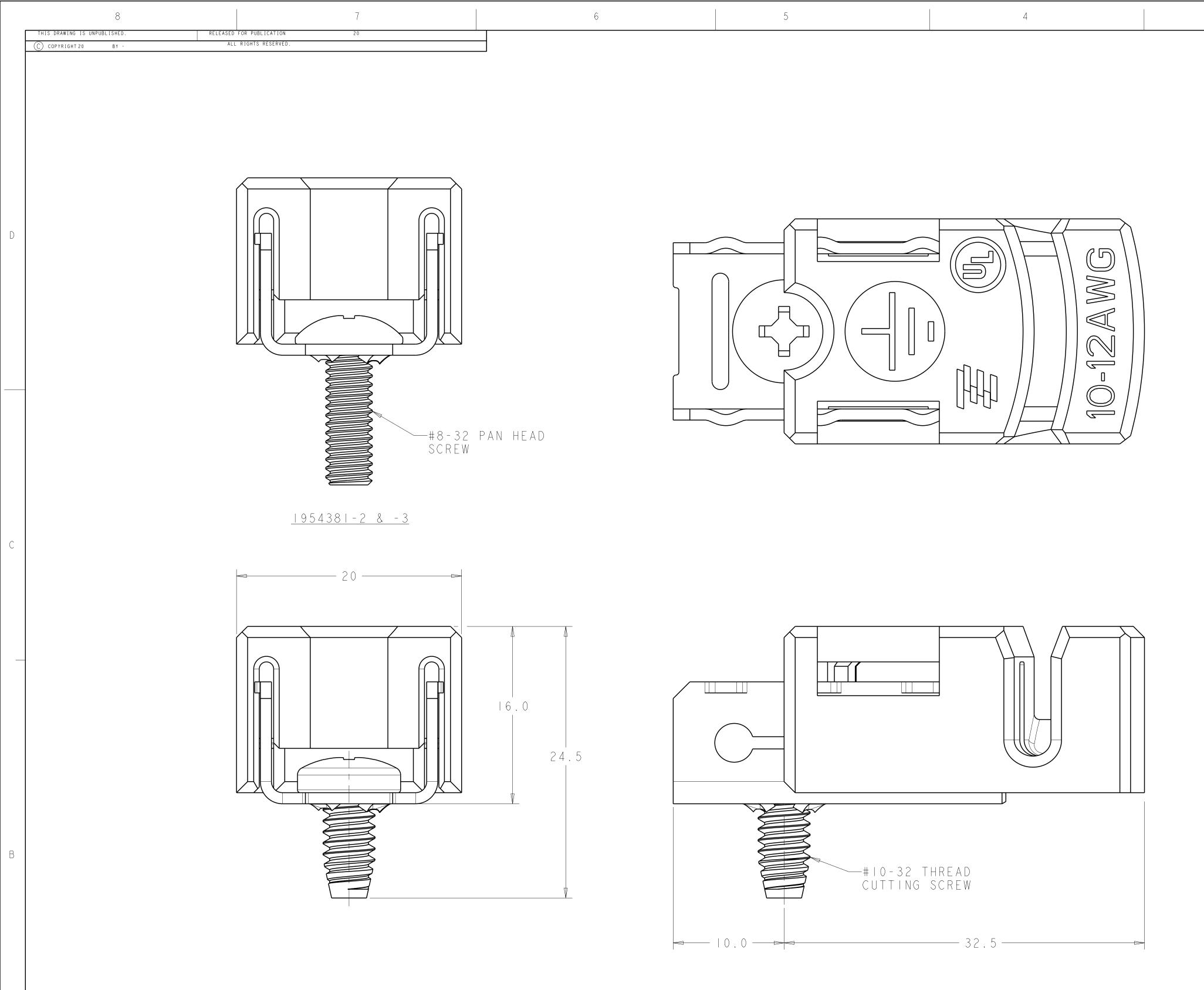
A MATERIALS AND FINISH: SLIDER: PBT, UV FI RATING, BLACK, 94V5 BASE: PHOSPHOR BRONZE; FINISH: Sn OVER Ni MOUNTING HARDWARE: STAINLESS STEEL EXCEPT #8-32 HEX NUT WHICH IS CARBON STEEL
