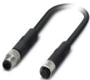
Sensor/actuator cable, 3-position, PUR, black RAL 9005, Plug straight M5, A-coded, on Socket straight M5, A-coded, cable length: 1 m
