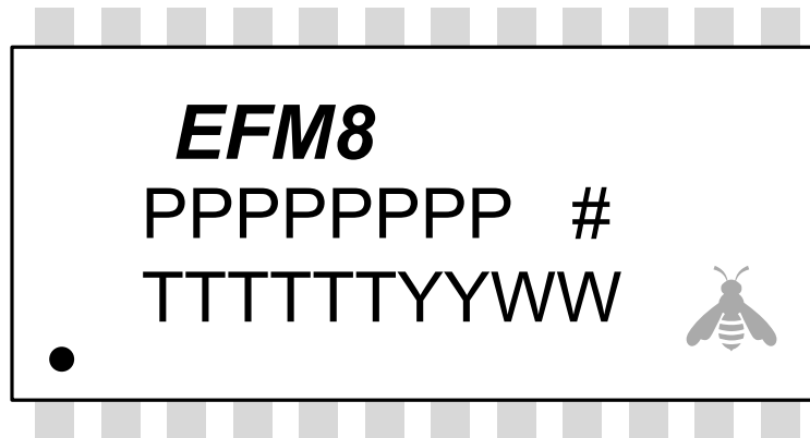
Figure 11.3. QSOP24 Package Marking
