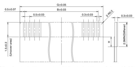
Note 1 : Stiffener dimension should be 2.5mm min., and H dimension should be 0.5mm for improved flexibility of FPC. Note 2 : When using the FPC/FFC in FH34S or FH19SC connectors, the exposed area inserted in either connector is 2.5mm  $\pm$  0.3mm and the stiffener is 3.5mm min.
