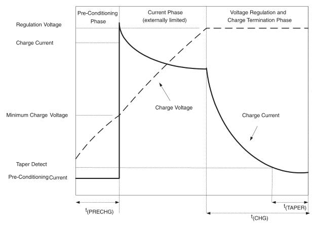
Figure 6. Typical Charge Profile
