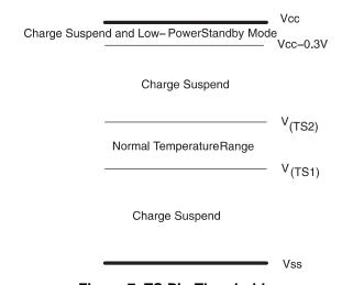
Figure 7. TS Pin Thresholds
