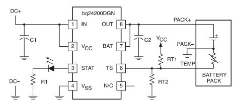
Figure 5. Low Dropout Single-Cell Li-Ion/Li-Pol Charger
