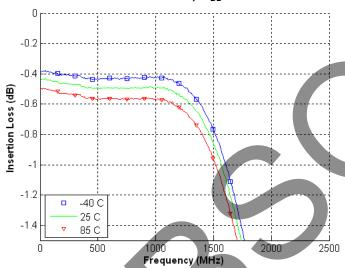
Figure 12. Rx Insertion Loss
