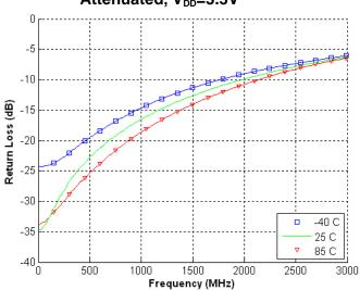
Figure 22. Rx Return Loss Attenuated, +25°C
