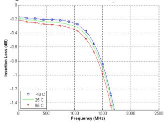
Figure 11. Rx Insertion Loss Un-Attenuated, V<sub>DD</sub>=3.3V
