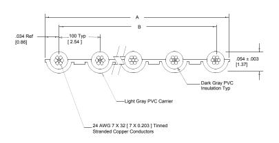
Note: Red marking on one edge of cable designates wire #1.
