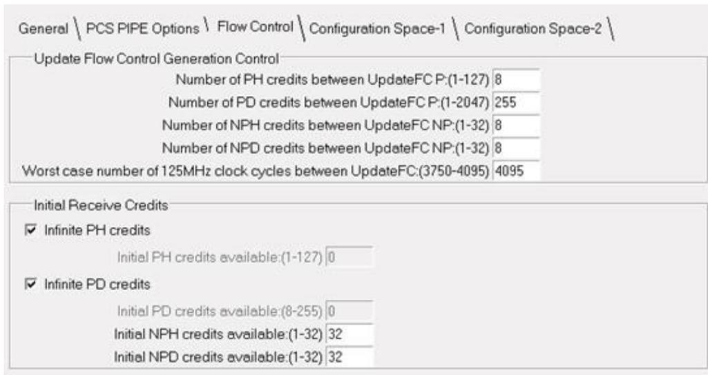
**Figure 3.3. PCI Express IP Core Flow Control Options**
