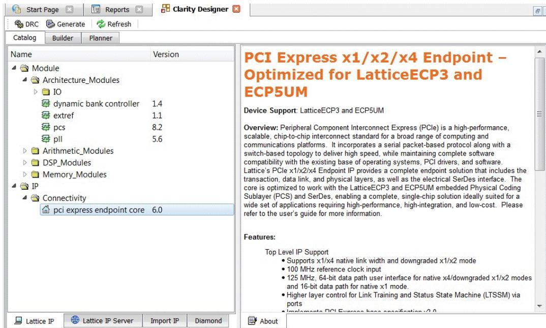
Figure 4.4. Clarity Designer GUI (pci express endpoint core)
