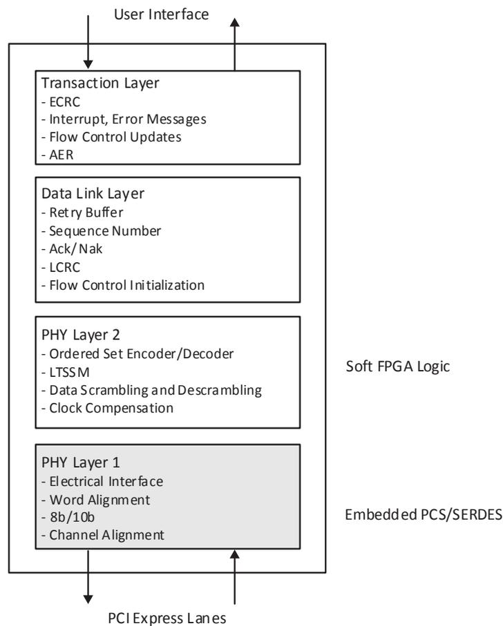
**Figure 2.1. PCI Express IP Core Technology and Functions**
