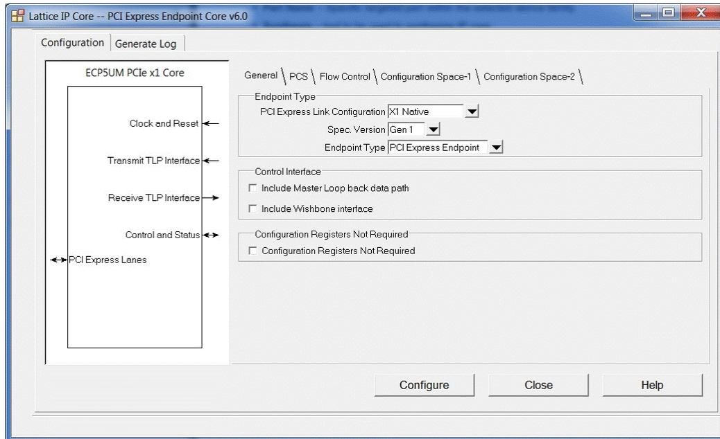
**Figure 4.6. PCI Express Endpoint IP Core Configuration GUI**
