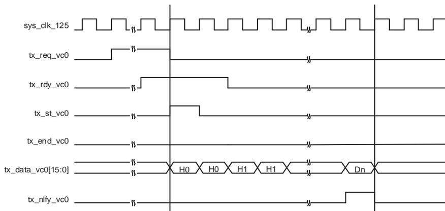
**Figure 2.15. Transmit Interface Native x1, Nullified TLP**
