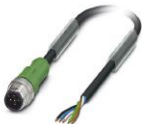
Sensor/actuator cable, 5-position, Variable cable type, Plug straight M12, coding: A, on free cable end, cable length: Free input (0.2 ... 40.0 m)
