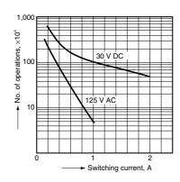
3. Contact reliability for AC loads Tested sample: DS2E-S-DC24V 10 pcs. Operating speed: 20 cpm. Detection level:  $200 \text{ m}\Omega$
