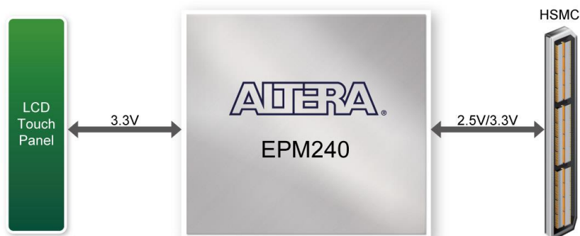
Figure 3-6 Block Diagram of the Bus Controller
